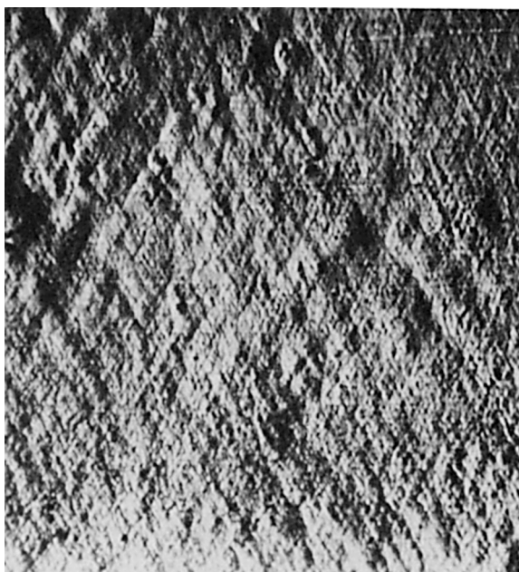
Fig. 11. Shear banding in homogeneously deformed plasticized (20 phr) PVC.
